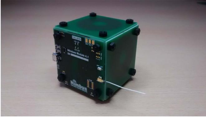
Fig. 13. Fully assembled module in cuboid form, with four PCB faces for planar coils, one for the electronics, and another for internal connectors.
