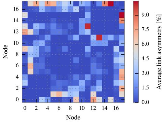
Fig. 6. Link asymmetry calculated as  $|PDR_{n \rightarrow m} - PDR_{m \rightarrow n}|$ .
